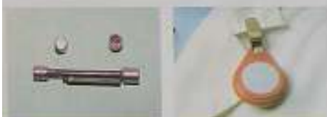
Fig. 2. Diffusive sampler for thermal desorption (ATD-50) and diffusive sampler for solvent desorption (SM-2000).
